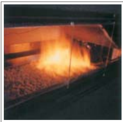
Some cellulose samples have failed the ASTM E970 fire safety test only six months after installation.
