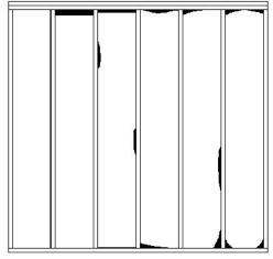
No more than 2% of surface area of insulation missing is acceptable for "Grade II"
