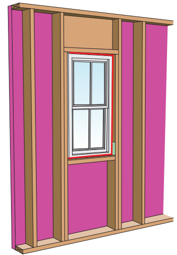
Figure A.2j: Air seal window around entire perimeter from interior with non- expanding foam.
